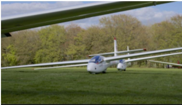
Pilots need to be aware that we winch launch gliders with cables which go up to theoretically 3700 ft QNH. That is unusual, but 2500 ft QNH is a normal height for a winch launch. A close encounter between a Dyneema winch cable and an aircraft would have a very bad outcome, both for the glider and the conflicting aircraft.
