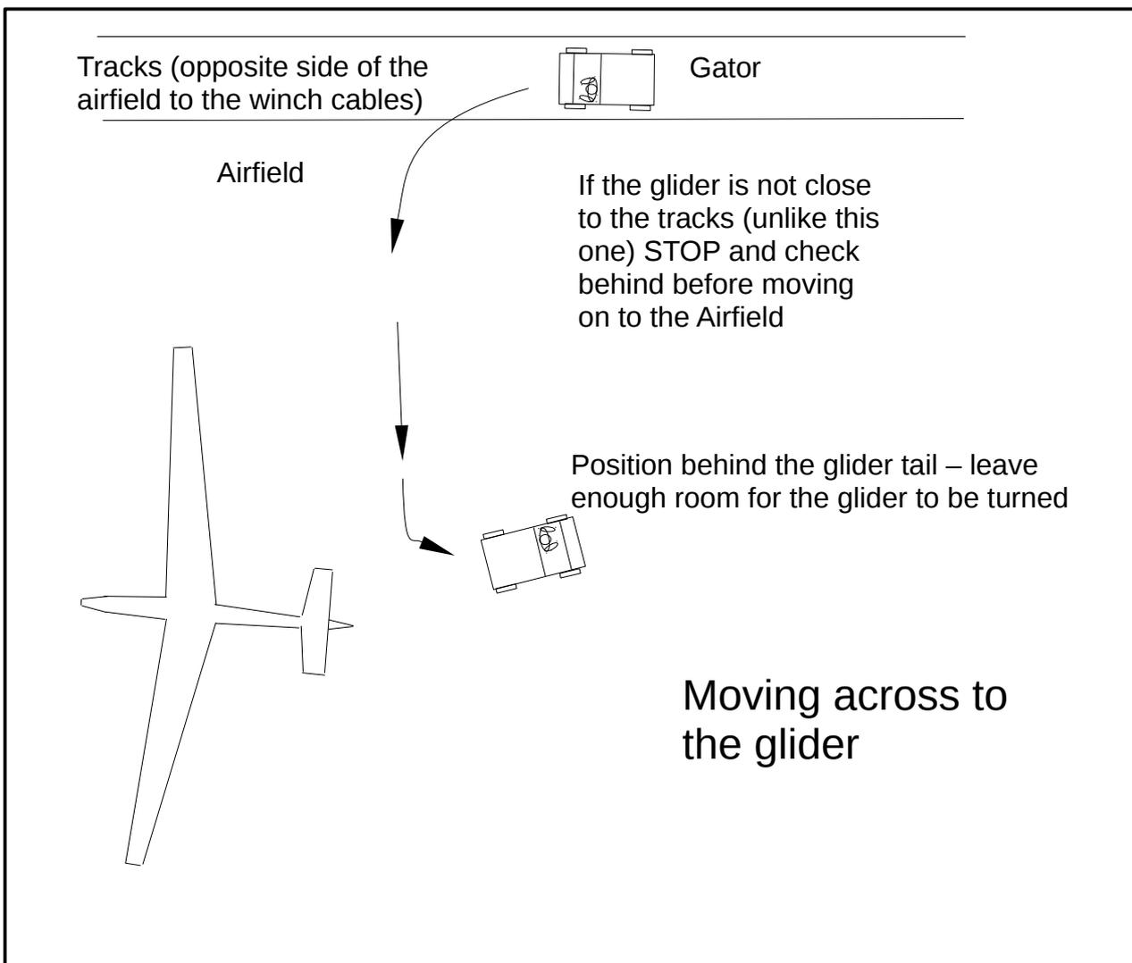
4. Using the L gear setting, set off down the airfield towing the glider, move as close to the tracks as you can. The wing tip holder will be on the airfield and the opposite wing of the glider will be overhanging the tracks and the adjoining field. Maintain a walking pace and frequently check behind that the wing tip holder is comfortable with the speed.
